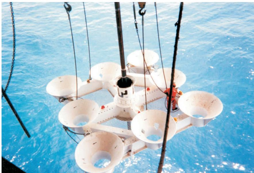
**Template used for pre-drilling project in the Rosetta gas field in the Nile Delta allowed completion of project in time to meet gas delivery dates. 4 wells were pre-drilled and 2 30-in. conductors set.**
