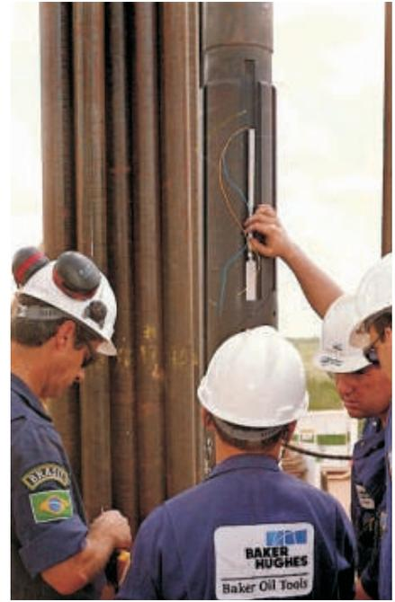
Installing and testing the world's first downhole electric wet-mateable connector system.
