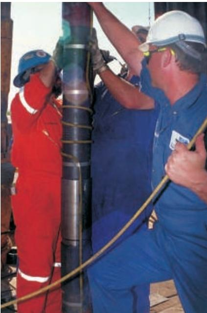
Baker Oil Tools technicians make up the world's first downhole electric wet disconnect tool.
