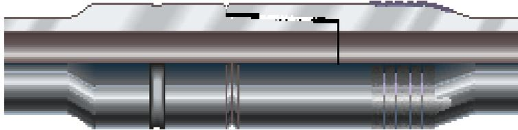
**Second-generation double-shoulder drill pipe connection provides increased torsional capacity, promotes more streamline configurations and tolerates more tool joint wear than standard API rotary shoulder connections.**
