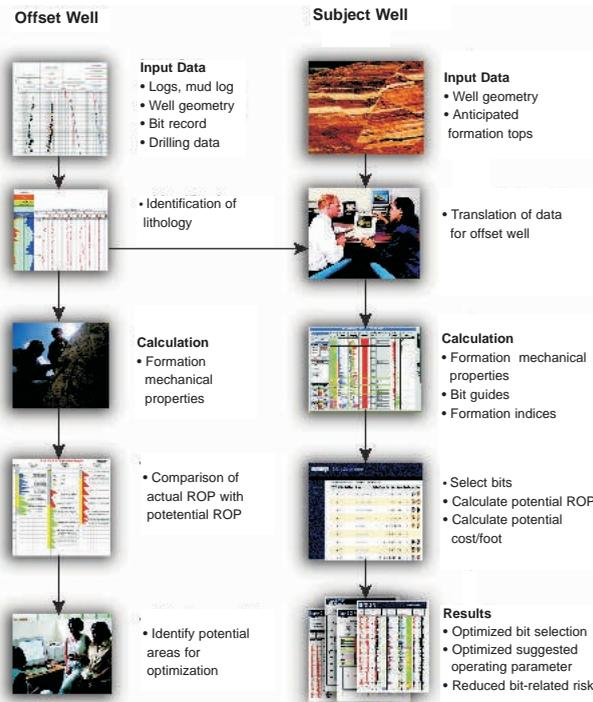
**Following a software-driven bit selection process when selecting the optimum bit series for a new well allows more accurate translation of offset data to the planned well and more comprehensive cost/risk/performance analysis of the wide range of bits.**
