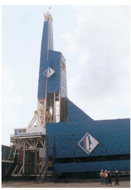
The Yastreb will drill extended reach wells from Sakhalin Island to offshore bottom hole locations six miles away. The rig is designed to withstand seismic events and temperatures as low as -40 degrees C.
