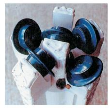
The Disc-Bit type cutter has been in use since the mid-1950s in tunnel boring applications.
