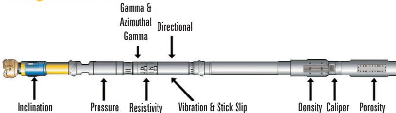
A higher level of integration with MWD/LWD systems allows positioning of LWD sensors closer to the bit while simultaneously minimizing BHA length and increasing reliability.
