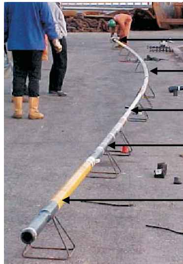
3-1/8" Mach 1 XL Motor (BHI) 3-1/8" Slimpulse MWD (Anadrill) 3-1/8" Resistivity Tool (TARGET) 3-1/8" Filter Sub (BHI) 3-1/8" Thruster (BHI)
