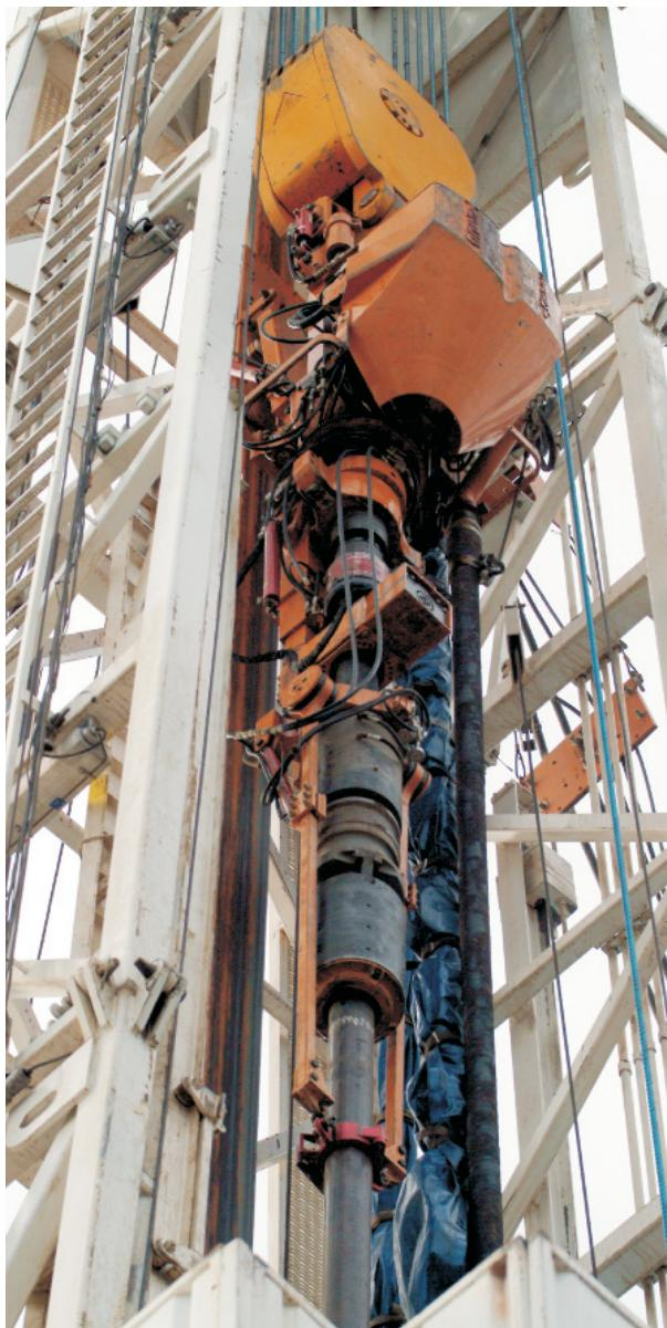
The Casing Drive System is installed directly into the rig's top drive drilling system after the drillpipe elevators, links and saver sub are removed. The CDS replaces power tongs, casing elevators, stabbing board, elevated work platform for tong operations, and fill-up tool.
