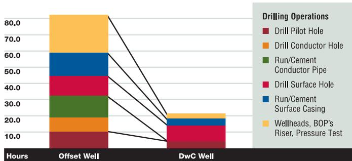
DwC uses a casing string that terminates in a special drill bit to drill and case a well simultaneously. Some areas of the world have used basic applications of the technology since as early as the 1950s.
