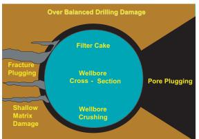
Damage to the reservoir during overbalanced drilling results from the influx of non-native fluids, chemicals and formation solids into the porosity of the formation.
