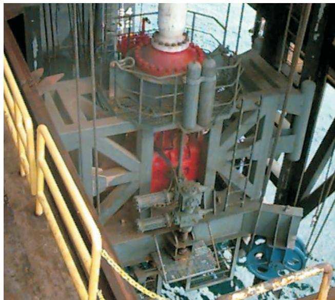
The recent conversion of Diamond Offshore's Ocean Baroness from a conventional subsea BOP to surface BOP configuration marks the fourth semisubmersible conversion by Unocal since 1996.
