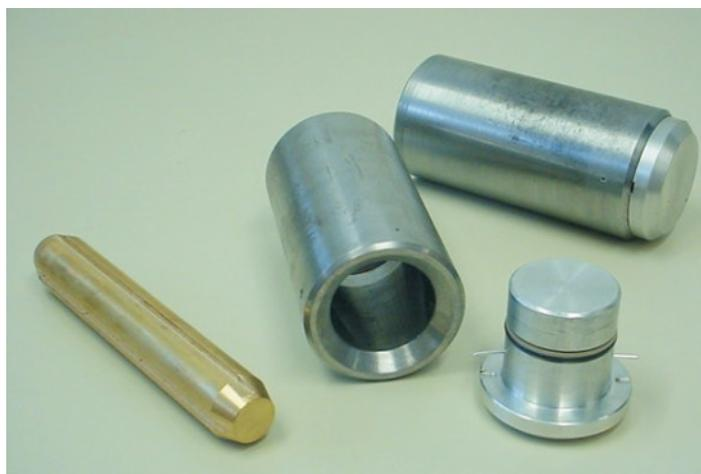
The components of the VDBP system. The new plug has one O-ring with a backup ring in an external groove on the plug. The O-ring seats inside a specially-built collar threaded on the end of the tubing. Two small shear pins help hold the plug in place while running in the well.
