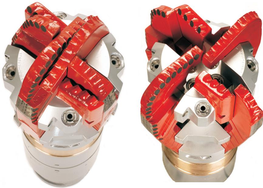
The expandable drill bit's closed configuration is shown on the left with the expanded mode on the right. During field tests with Unocal in Indonesia, weight on bit required to achieve a specified controlled penetration rate was 39% lower than for offset tricone runs.
