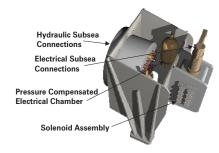
A newly patented electro-hydraulic (EH) control system has been developed that can be retro-fitted to existing installed all-hydraulic subsea control systems, utilizing the existing driller's and toolpusher's panels, pump/accumulator unit, UPS, most of the rig's wiring and both subsea pods. IADC/SPE 87156
