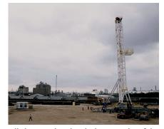
With the substructure in the low position, the mast is pinned to the middle drill floor section. The mast cylinders are pinned to the lower section of the mast and then hydraulically telescoped. With the mast in the vertical position and the hydraulic raising cylinders still in place, mast support legs are swung out and pinned to the floor. The mast-raising cylinders are then disconnected and retracted.
