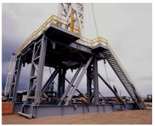
The drill floor is then hydraulically raised via the telescoping cylinders. Telescoping braces prevent the substructure from rotating past the vertical position. The braces are extended when the floor is at ground level, and as the substructure rises, the braces retract and "bottom out" on a stop and are secured with pins.
