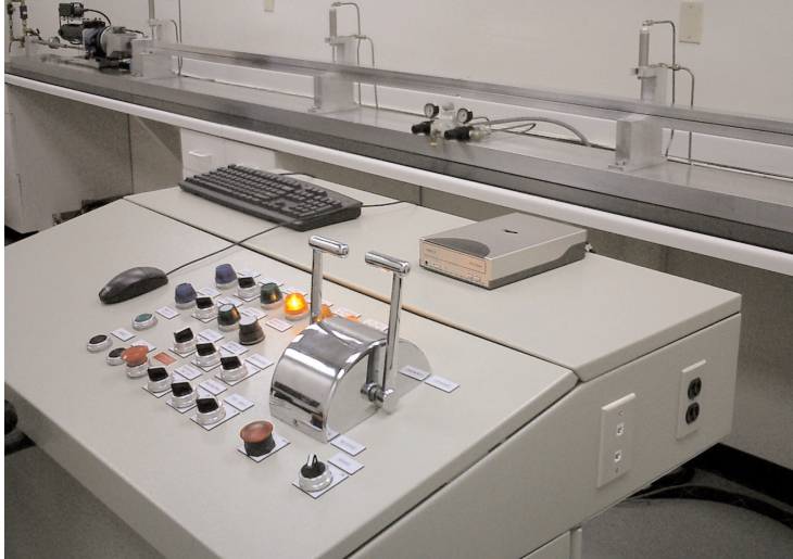
Slider built a laboratory model to test the automation system that was comprised of three basic components for simulating the surface controls, wellbore events and downhole conditions.
