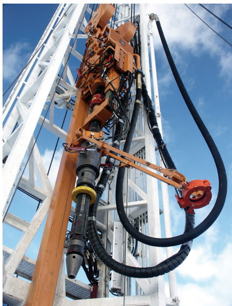
The portable casing drive system attaches to the top drive to facilitate Casing Drilling and casing running operations.
