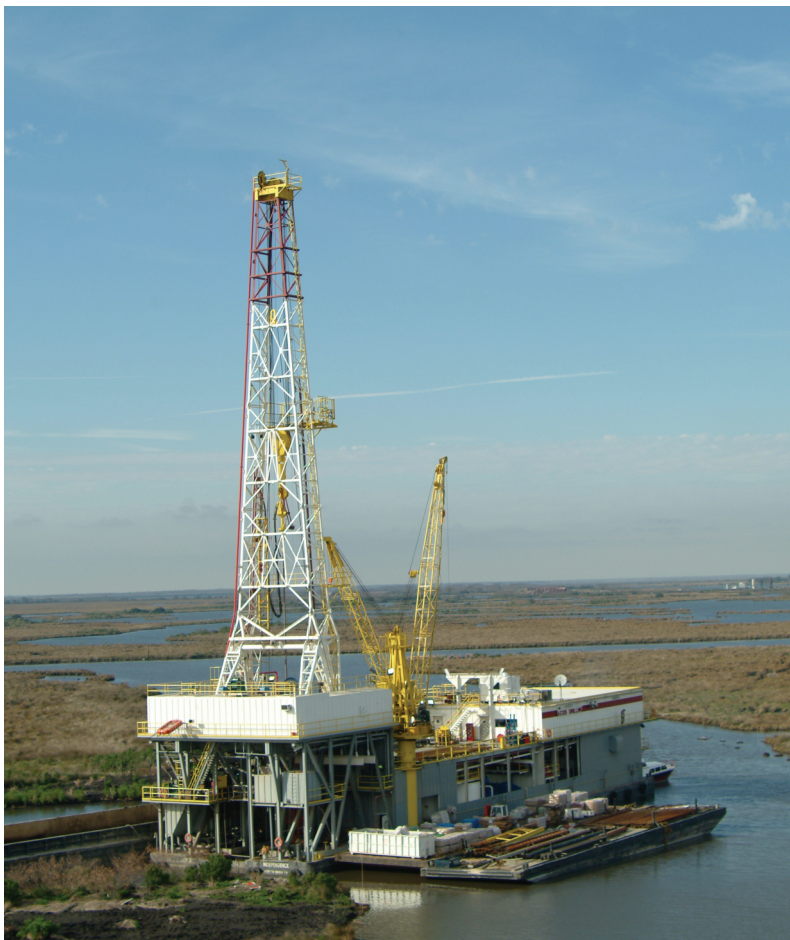
Axxis' inland water drill barge Independence features circular mud tanks, high capacity cranes and the latest technology in remote monitoring to view virtually any operating parameter remotely in real time.
