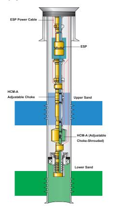
An example of a "typical" intelligent completion with commingled production from two zones with adjustable chokes and artificial lift provided by en electric submersible pump.
