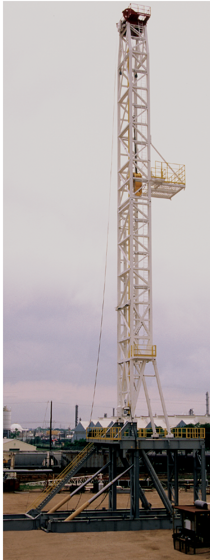
National Oilwell's Ideal 1500 rig requires only about 15 minutes to raise and pin the rig floor and the mast once they are in place at the rig.
