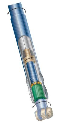
The steering section assembly of the Power-Drive Xceed continuously orients the tilted shaft to control the drilling directions and the dogleg severity of the borehole.
