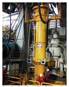
Use of a silicate-base drilling fluid in tandem with a unique mud recovery system combined to stabilize a problematic formation in the West Azeri field in the Caspian Sea. SPE/IADC 92769.
