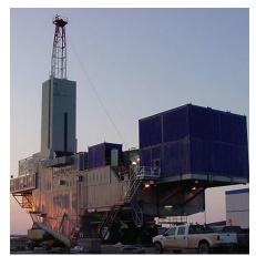
Combining coiled tubing drilling technology with a conventional jointed pipe workover capability represents the next step change in providing low-cost reserves access via the most efficient tool for the application. SPE/IADC 92207.
