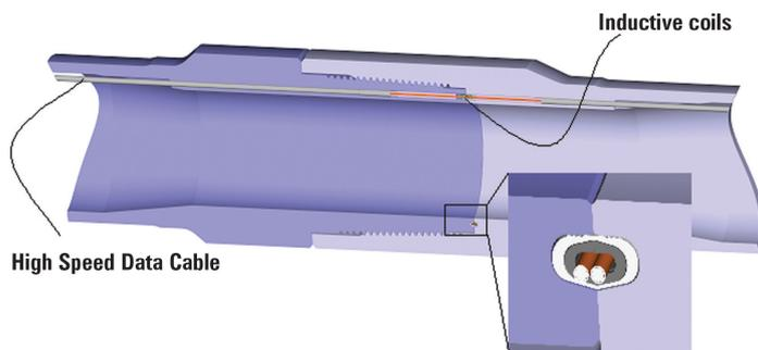
**Drillstring components capable of transmitting data at rates up to 2 megabaud have been developed and successfully tested in commercial drilling applications. The new technology can improve well productivity and reduce drilling time. SPE/IADC 92477.**
