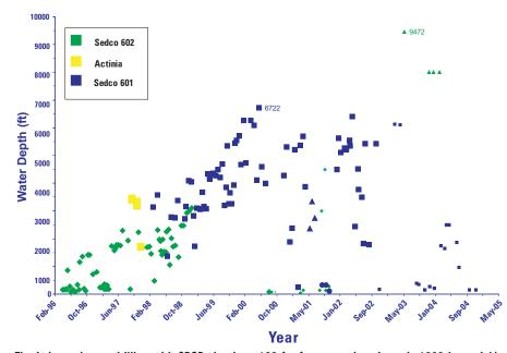
The industry began drilling with SBOPs in about 100 ft of water or less in early 1996 but quickly moved into ever increasing water depths, including several wells in water greater than 8,000 ft and one approaching the 10,000 ft water depth mark. Chart courtesy of John Kozicz, Transocean.
