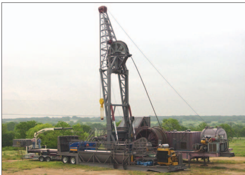
A field demonstration of a microhole coiled tubing drilling rig shows its small footprint. Some can be mounted on a trailer pulled by a standard pickup truck.
