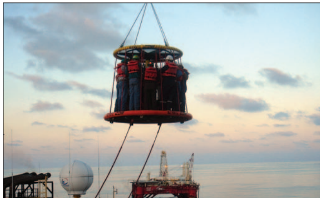
For BP's Thunder Horse project, Billy Pugh Co. developed the 12-person version of its X-904 personnel transfer device to move more than 500 people a day.
