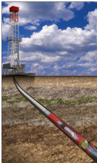
**In the 100th installation of the downhole deployment valve, Weatherford installed a 7-in. DDV through 9 5/8-in. casing landing in open hole in the North Sea.**
