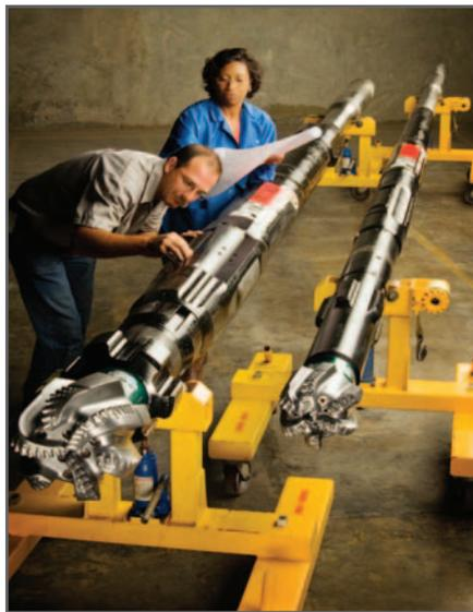
**The 12 ¼-in. PathMaker rotary steerable system has drilled more than 290,000 ft of hole in areas such as Gulf of Mexico, US land, the North Sea and the Middle East. Recently the system was used onshore Egypt and was able to eliminate a hole-opener run.**
