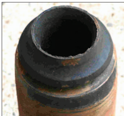
Figure 4: This photograph of a pin tool joint failure shows a blackened carbon deposit on the OD and ID surfaces, indicating high heating occurred at the failure location.
