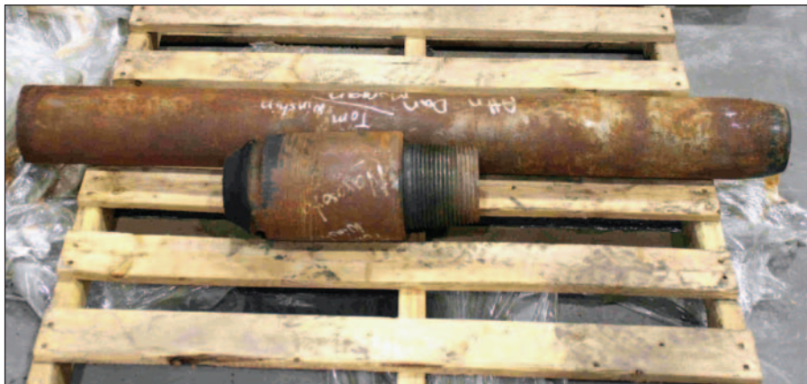
Figure 3: Drill pipe and drill stem failures caused by downhole frictional heating are becoming more common. The exaggerated necking at the failure location on this pipe section required heating while axial tension was applied.
