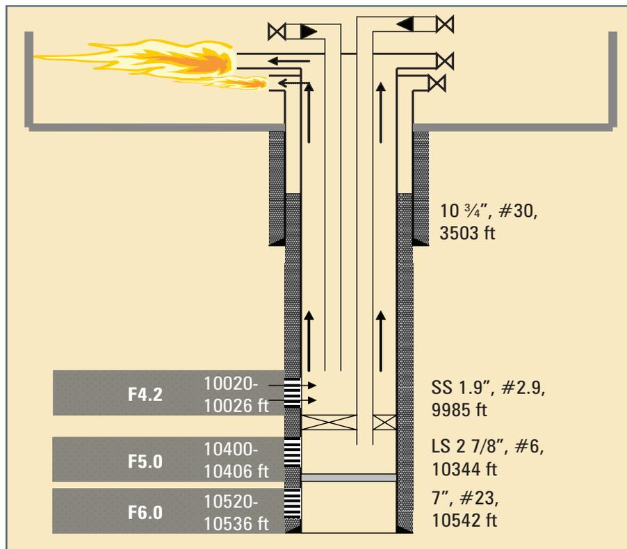
**This schematic shows the blowout situation after an illegal oil bunkering incident on the mainland of the eastern Niger Delta. In such bunkering cases, no records on flow, pressure, produced fluids, etc., are available. With considerable uncertainty, the kill design had to take into account any possible combination of critical factors to ensure that once the kill starts, it could be concluded successfully.**
