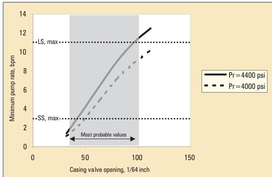
**It was estimated that the casing valve opening was between ½ in. and 1 ¾ in. For the range of formation pressure and casing valve openings, required pump rates to kill the well were determined to range from less than 2 bpm for the smallest opening of the casing valve and reduced formation pressure to as much as 12 bpm for a 1 ¾-in. open casing valve and full hydrostatic pressure.**
