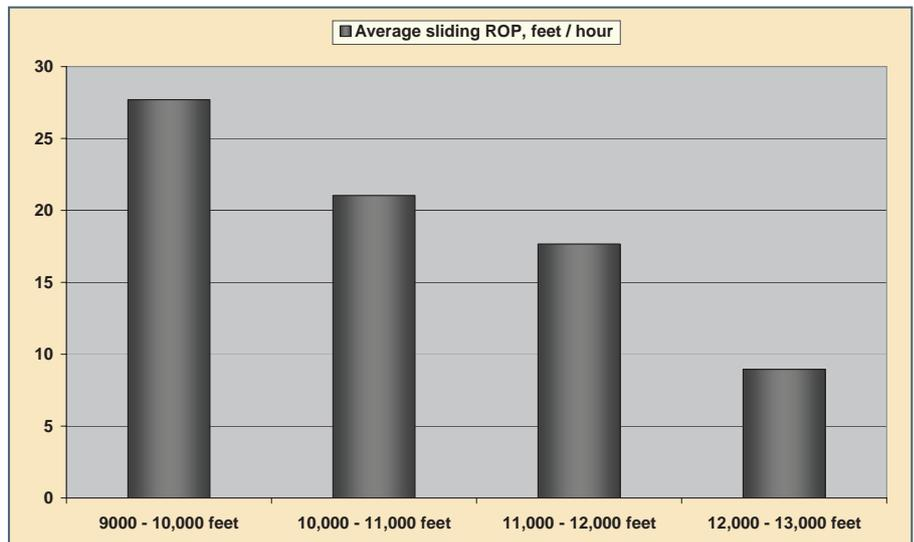
**Figure 4 shows that in the conventionally drilled wells offshore Libya, ROP while steering — when the drill string was sliding rather than rotating — decreased significantly with depth due to increasing drag on the drill string.**
