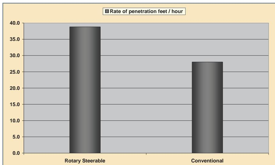
**Figure 5 shows that 3 wells using rotary steerables drilled 38.6% faster than the 4 conventionally drilled wells offshore Libya in the Mediterranean.**
