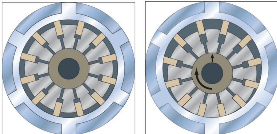
**Figure 1: Neutral position (above left): Drive shaft concentric with non-rotating sleeve. Steering position (above right): Drive shaft deflected from center line of hole.**
