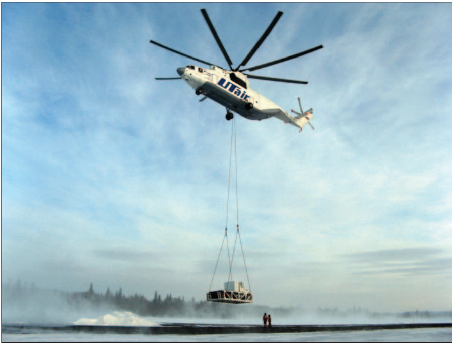
The Russian MI 26 helicopter, the largest in the world with a lifting capacity of 44,000 lbs, flies a wheeler truck to a Nabors universal transport container. Nabors is currently building heliportable rigs to increase access to remote areas.
