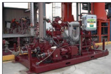
THE SECURE Drilling System is a closed-loop system that analyzes available drilling data to detect kicks or losses and automatically manages backpressure at the surface to control influxes or losses. The system allows the volumes to be kept as small as possible — a micro-influx or micro-outflux. The system is designed to incorporate existing drilling and pressure control equipment with minimal upgrades and equipment additions.
