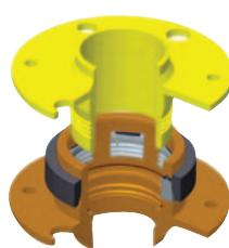
**VETCO GRAY'S NEW** marine riser system, the MR-6H SE, combines field-proven technology of the H-4 subsea wellhead connector and the dog-style marine riser (MR). To make the fully automated connection of the MR-6H SE, hydraulic units on the spider engage a cam ring on the box, which actuates 6 dogs into the profile in the pin. This creates a full pre-loaded connection with an efficient and effective load path.
