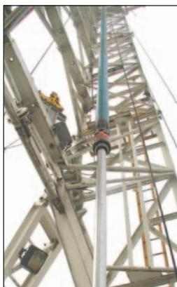
**BAKER OIL TOOLS'** linEXX Solid Expandable Monobore Liner Extension System optimizes casing configurations for drilling deeper or isolating trouble zones without reducing critical hole size. The system consists of the RC9 series casing shoe, FORMlock expandable liner hanger/packer, linEXX solid expandable casing, RNX retrievable guide shoe and catEXX hydraulic, top-down expansion system.
