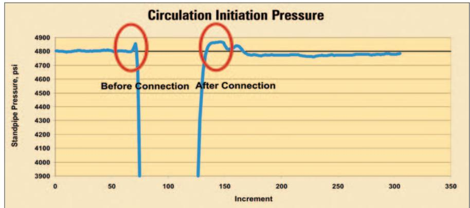
**Above:** With its constant, low-energy gel structure, pressure spikes associated with initiating circulation are virtually eliminated with the RHEO-LOGIC system. **Below:** Surge pressures when running casing with the RHEO-LOGIC system are reduced when compared with conventional SBM, resulting in minimized downhole mud losses.
