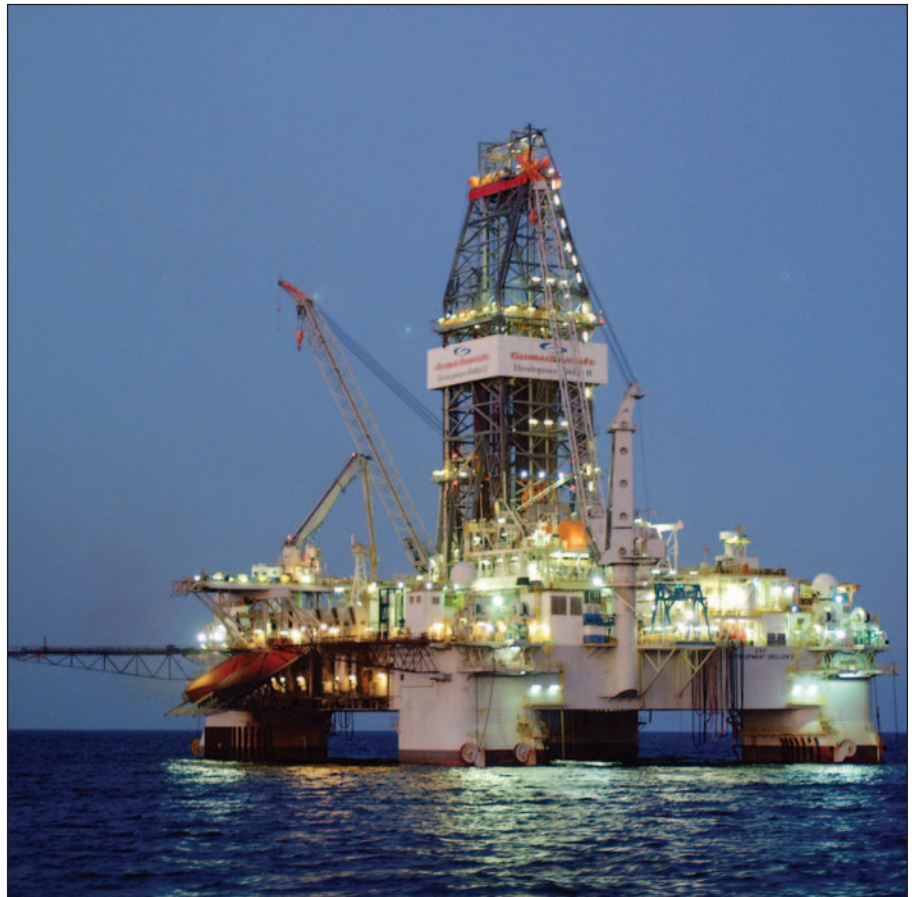
GlobalSantaFe's Development Driller class units were designed for complex deepwater developments. The Development Driller II, seen above, commenced operation in November 2005 and has been drilling and completing wells that were previously batch set.
