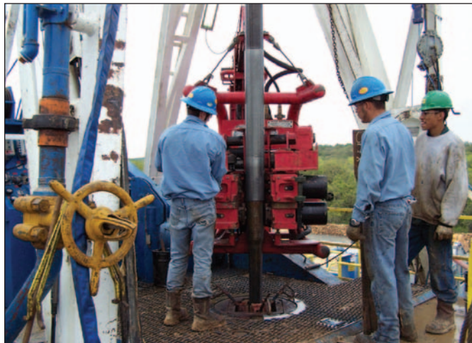
Bandera Drilling recently installed an Iron Derrickman on Bandera Rig 7. The West Texas area is experiencing some slow-down, said Ray Brazzel, president of the Abilene-based company.
