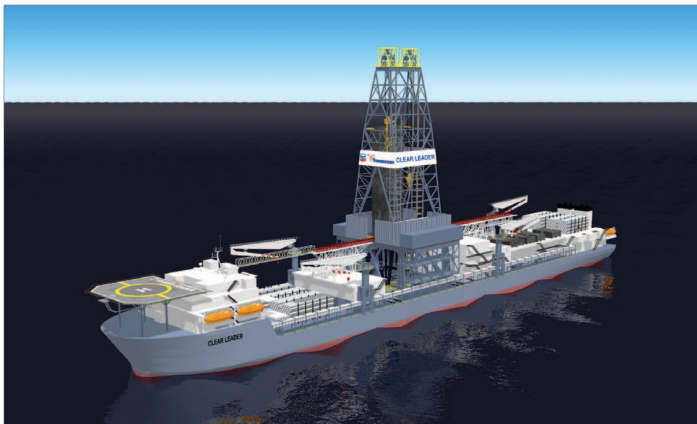
A computer-aided rendering of Transocean's Enhanced Enterprise class drillship Discoverer Clear Leader shows the dual-activity derrick, with stands of pipe made up offline in one derrick while drilling ahead with the second derrick.
