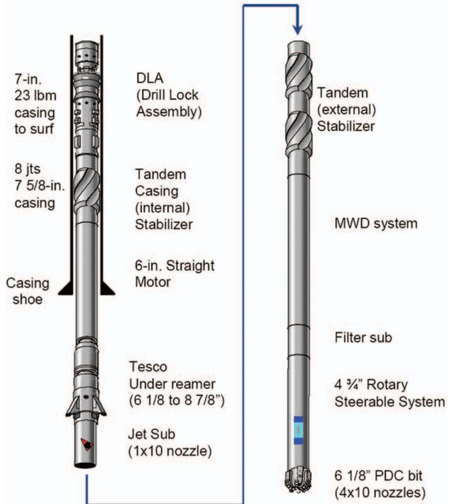
The BHA for casing directional drilling with a rotary steerable system for Well 91 was 112 ft long with 85 ft stick-out below the shoe of the 7-in. casing.
