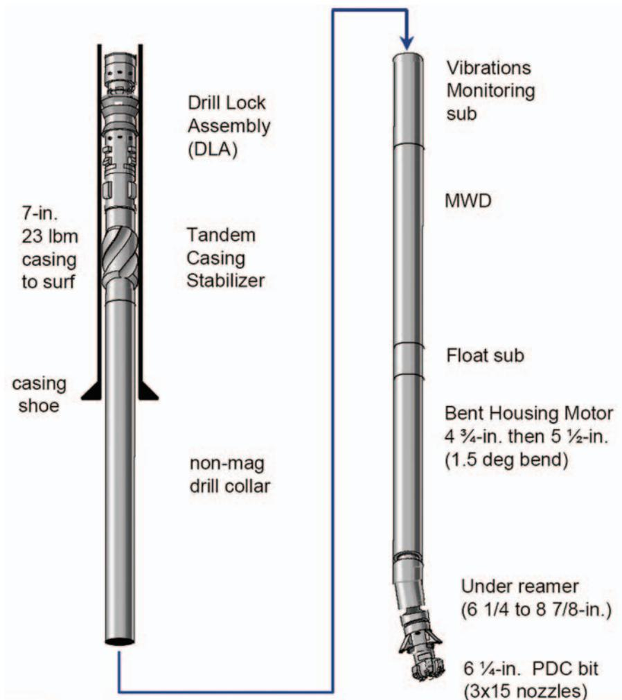
The bottom hole assembly with steerable motor above was used to casing directionally drill Well 83 in the Lobos field for ConocoPhillips. The assembly was positioned on the shoe joint of casing so that all components below the tandem stabilizer extended into the open hole below the casing.
